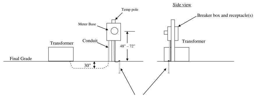
8' ground rod, clamp and #6 bare copper ground wire (Supplied and installed by consumer) Grounding conductor shall be connected from the ground lug in meter base to the ground rod(s) Copperative requires the meter base to be grounded
