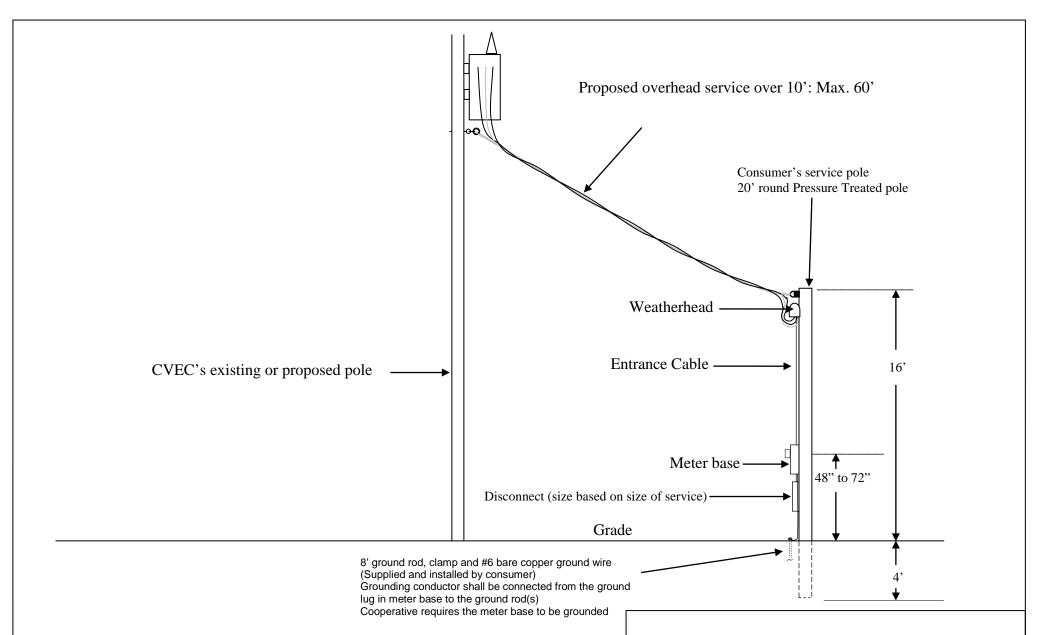
Consumer to provide all materials on the service pole, including the service pole. CVEC to provide the meter base (200 Amp or larger) and meter.
